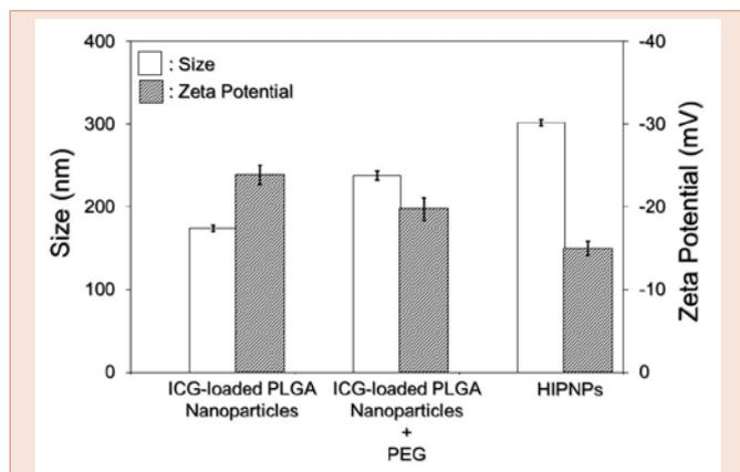
**Figure 3:** Quantitative analyses of the sizes (left Y-axis) and surface charges (right Y-axis) of the bare ICG-loaded PLGA nanoparticles, ICG-loaded PLGA nanoparticles coated with hetero-bifunctional PEG, and HIPNPs. Values are mean  $\pm$  SD ( $n = 3$ ).
