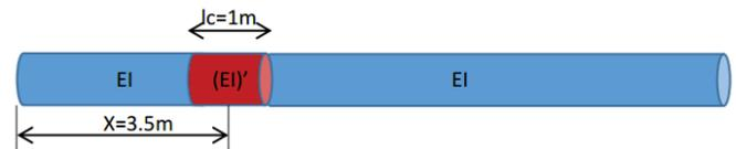
Figure 6: Finite element model.
