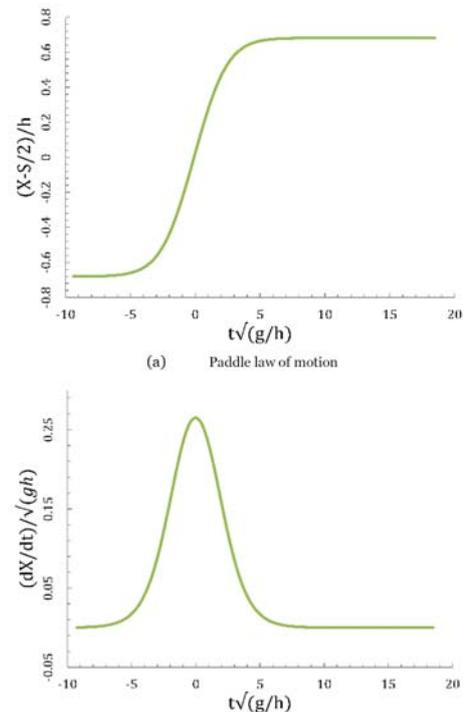
Figure 6: Paddle motion for  $E = 0.2$  and a water column of  $h=0.3$  m
