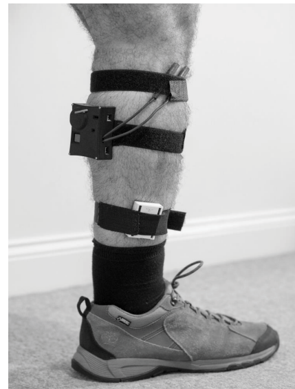
Figure 1: Image to show haptic device and vibrotactiles (without gait analysis markers in situ). The haptic device is the black box on the posterior calf. The vibrotactiles are shown positioned on the lateral aspect of the lower leg below the knee.
