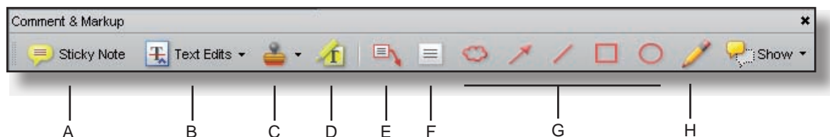
A. Sticky Note tool; B. Text Edits tool; C. Stamp tool; D. Highlight Text tool; E. Callout tool; F. Text Box tool; G. Various Object tools; H. Pencil tool
