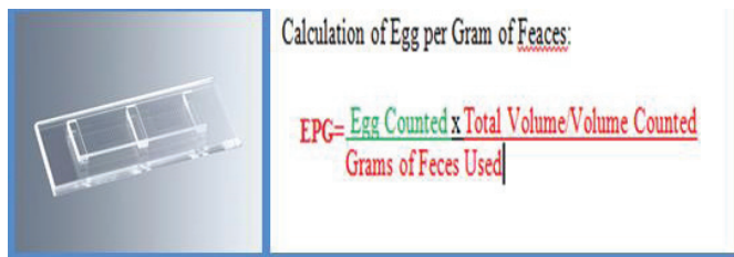
Figure 3: Macmaster two chamber and equation for egg per gram of faeces.
